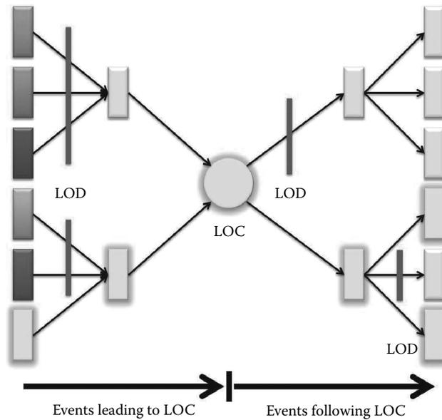
**FIGURE 15.4** (See color insert.) Bow tie model. LOC, LOD.
